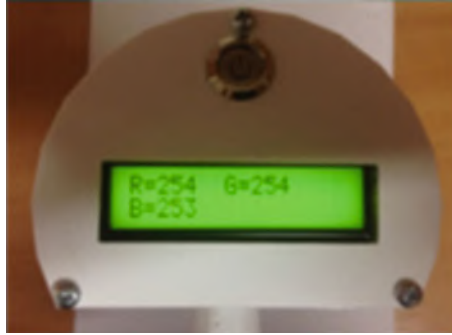
Fig. 1 The sensor was connected to LCD display and to the Arduino development board to show values of RGB directly on LCD display in real time
