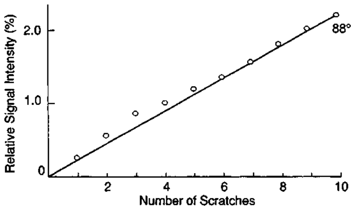
Figure 11-17 Experimental results for measurement of surface finish. (From T. Sawatari, Appl. Opt. 11, 1337 (1972).)
