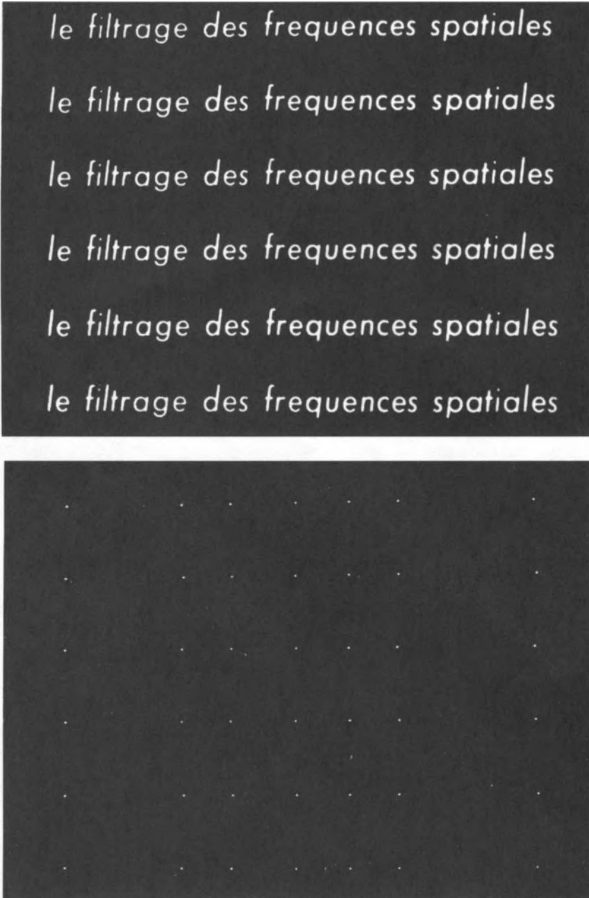
Figure 24-13 Identification of the letter e . The input is shown at top. Identification of the locations of the letter e are indicated at bottom by spots of light. (From S. Lowenthal and Y. Belvaux, Opt. Acta 14 , 245 (1967).)
