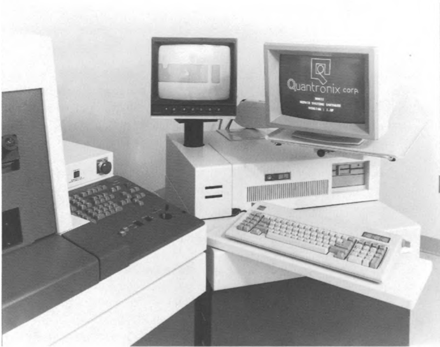
Figure 17-5 Production system for location, identification, and repair of photomask defects. The system can both remove excess metallization and fill in missing metallization. (Photograph courtesy of Quantronix Corp.)
