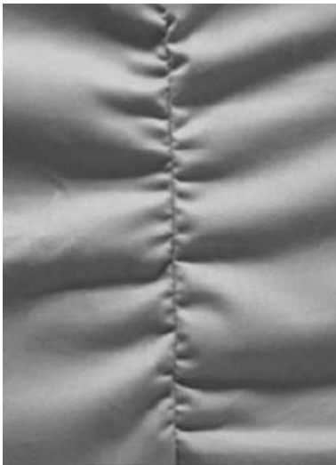
16.8 Pucker due to structural jamming.
