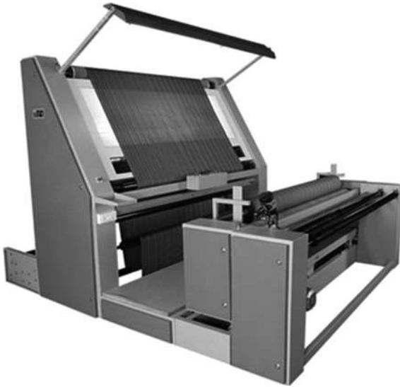
11.3 Fabric inspection unit.
