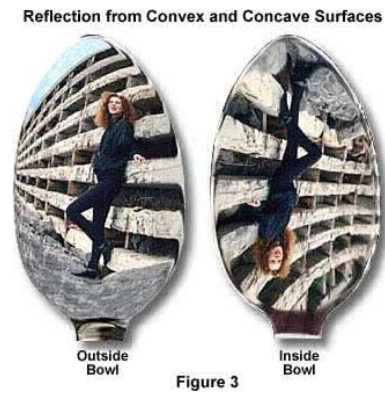
Figure 47.2: Types of mirrors, as illustrated in a table spoon. Left : The bottom of a spoon forms a convex mirror. Right : The top surface of a spoon forms a concave mirror. (Credit: Florida State University.)
