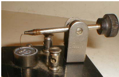
Figure 45.2: A galena crystal with cat's whisker. (©GNU-FDL, Wikimedia Commons.)
