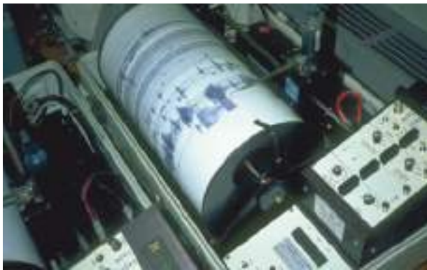
■ FIGURE 10.1 Seismographs record earthquake waves for scientific study.
