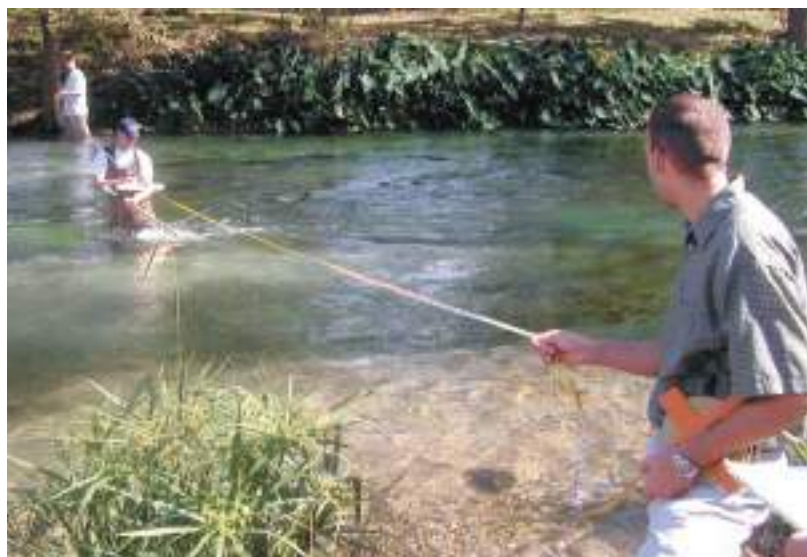
■ FIGURE 14.10 These university students are measuring a stream’s velocity, depth, and width in order to find discharge, the volume flowing in a stream per unit time.
