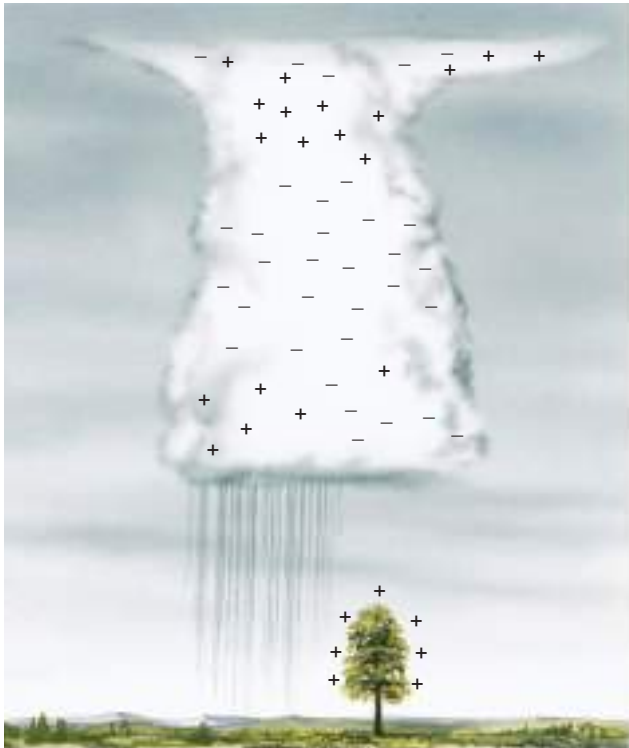
■ FIGURE 6.17 A cross-sectional view of a thunderstorm showing the distribution of electrical charges.
