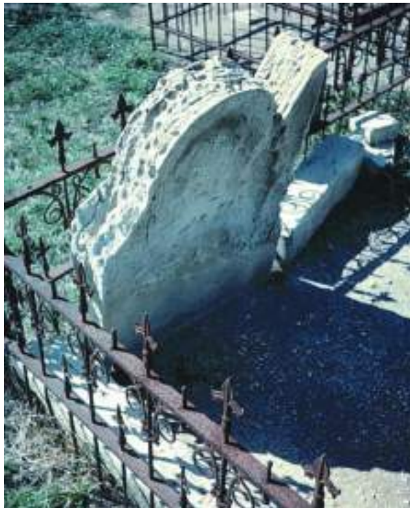
■ FIGURE 12.16 These limestone tombstones have undergone extensive chemical weathering, accelerated by air pollution.
