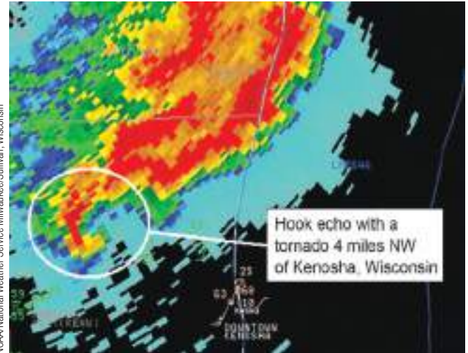
■ FIGURE 6.22 This Doppler radar image near Kenosha, Wisconsin, shows a curving pattern in the precipitation patterns of the oncoming storm, called a hook echo, which means a tornado may be developing.
