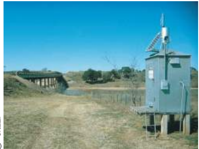
■ FIGURE 14.29 U.S. Geological Survey (USGS) stream gaging station. (a) As illustrated here, when river level rises or falls, so does the water in the lower part of the station, connected to the channel by intake pipes. A gaging float moves up and down with the water level, and this motion is measured and recorded. Gaging stations electronically beam flow data to a satellite that transfers the information to a receiving station. (b) Gaging stations are commonly located where highway bridges cross rivers or streams.
