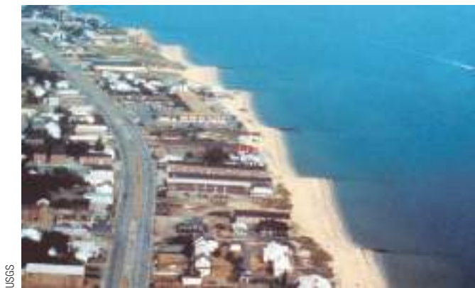
■ FIGURE 17.20 A series of groins on the Atlantic shoreline at Norfolk, Virginia, captures sand to maintain the beach along one stretch of the coastline.
