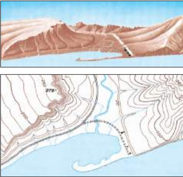
■ FIGURE 2.23 (Top) A view of a river valley and surrounding hills, shown on a shaded-relief diagram. Note that a river flows into a bay partly enclosed by a sand spit. The hill on the right has a rounded surface form, but the one on the left forms a cliff along the edge of an inclined but flat upland. (Bottom) The same features represented on a contour map.
