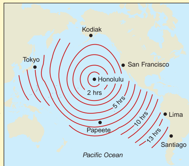
The Pacific Tsunami Warning Center locates earthquake epicenters and estimates arrival times for potential tsunamis in the Pacific region.
