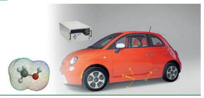
This battery-powered electric car is equipped with a methanol fuel cell that recharges the battery while the vehicle is driven. The methanol in the fuel cell is not burned but converted electrochemically through the use of a catalyst to carbon dioxide and water. The process produces an electric current that charges the battery.
