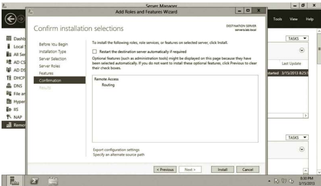
Figure 9.24 Confirming installation selections.
