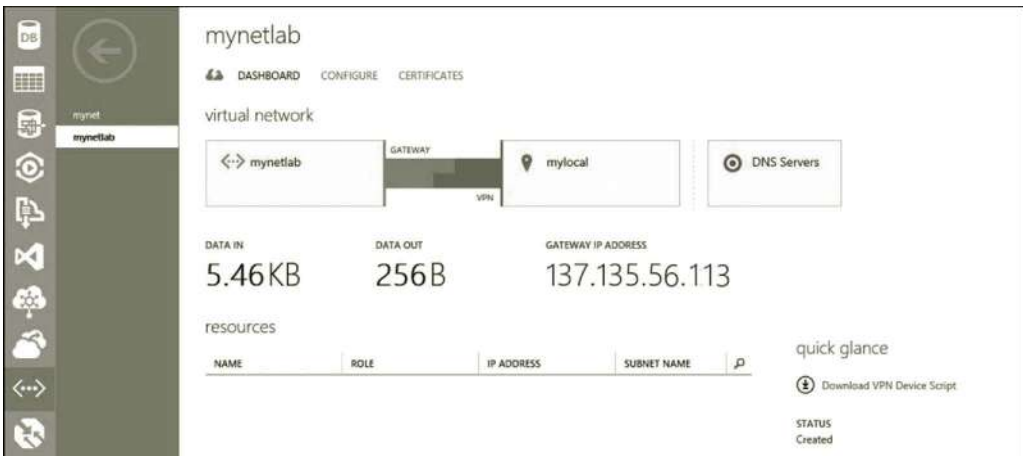
Figure 10.50 Established site-to-site connection.
