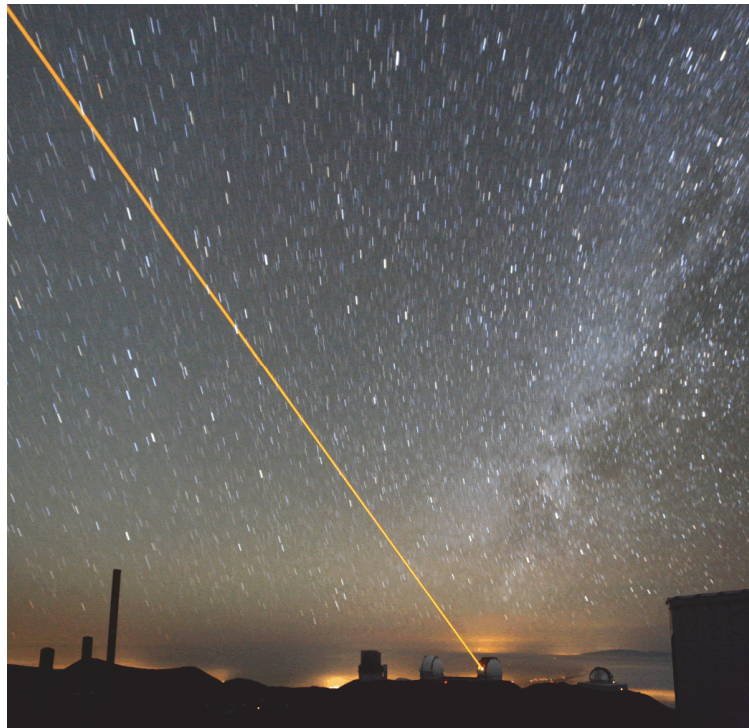
Figure 3-40 Laser guide star from the Keck-2 telescope on Mauna Kea, Hawaii. The stars moved noticeably during the three-minute exposure needed to record the laser beam.
