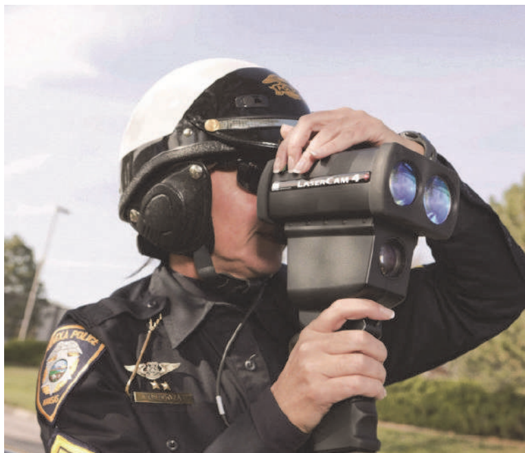
Figure 10-7 Applications for laser range finders. (Courtesy of Kustom Signals).
