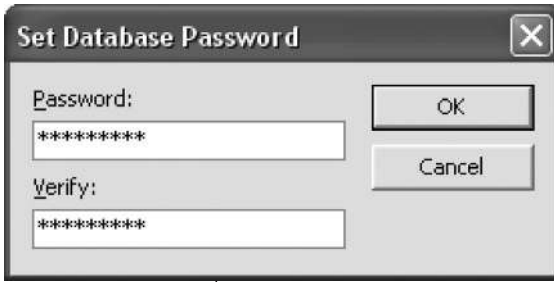
Dialog box to set a password to control access to the database (password not echoed on the screen)
