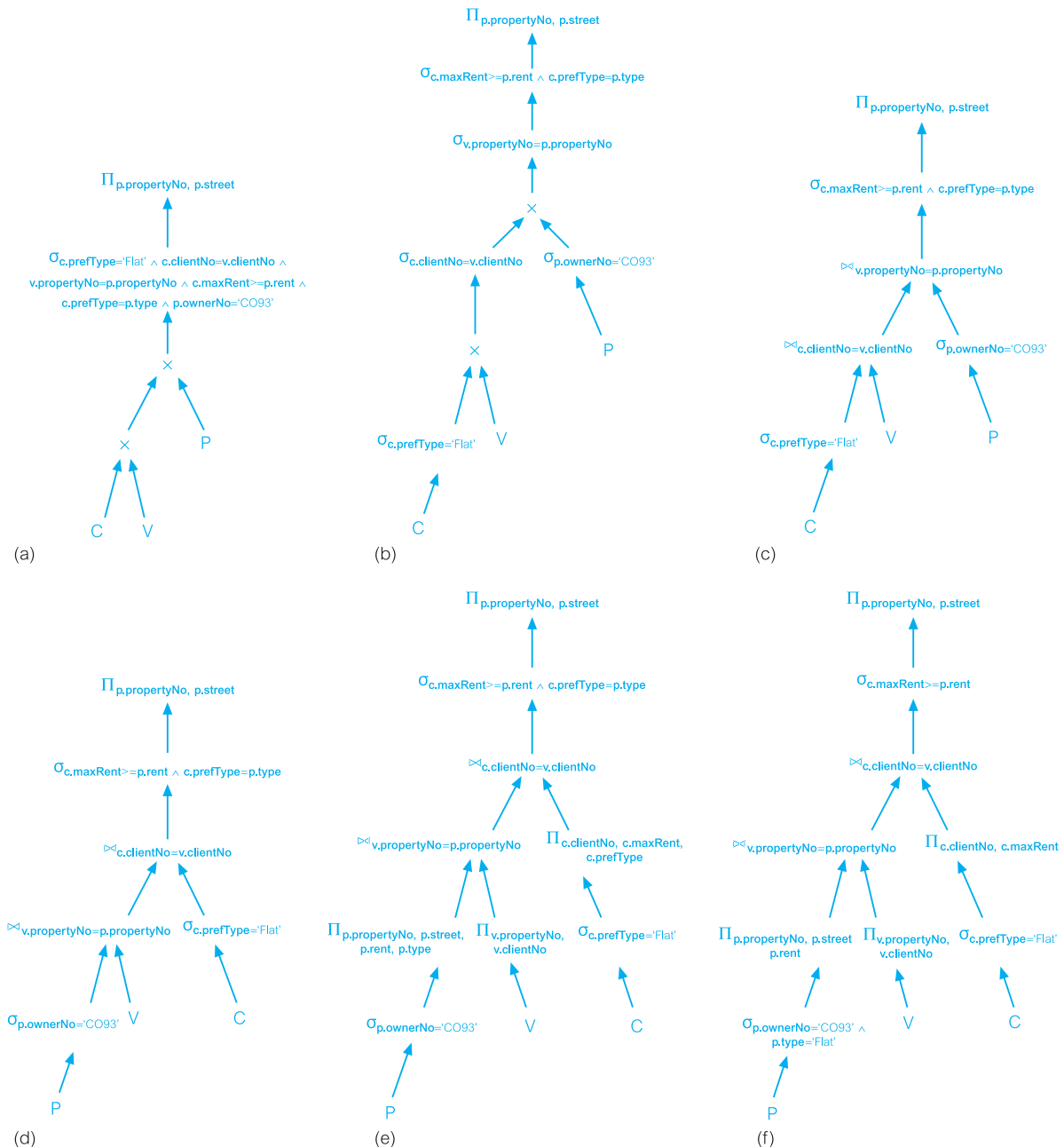
Figure 21.4 Relational algebra tree for Example 21.3: (a) canonical relational algebra tree; (b) relational algebra tree formed by pushing Selections down; (c) relational algebra tree formed by changing Selection/Cartesian products to Equijoins; (d) relational algebra tree formed using associativity of Equijoins; (e) relational algebra tree formed by pushing Projections down; (f) final reduced relational algebra tree formed by substituting c.prefType = 'Flat' in Selection on p.type and pushing resulting Selection down tree.
