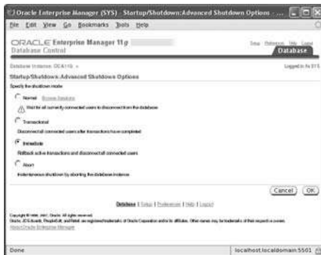
FIGURE 9.39 The Startup/Shutdown: Advanced Shutdown Options screen
