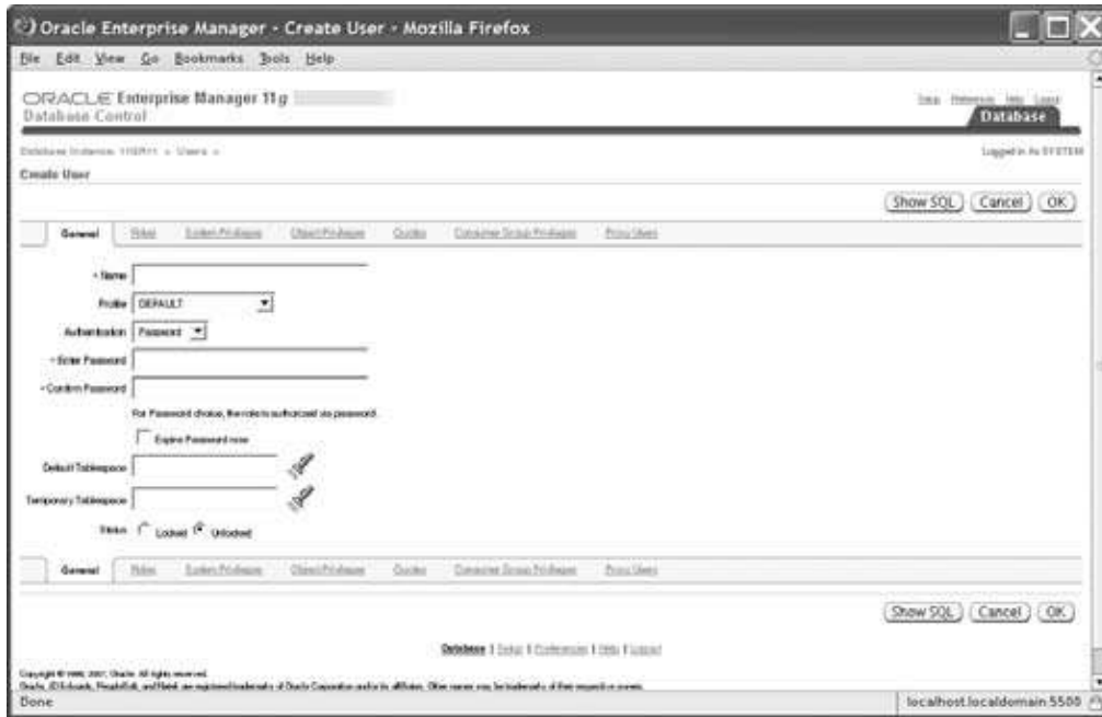
FIGURE 12.2 Grid Control's Create User screen
