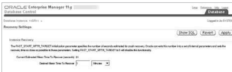
FIGURE 16.1 Adjusting MTTR for instance recovery
