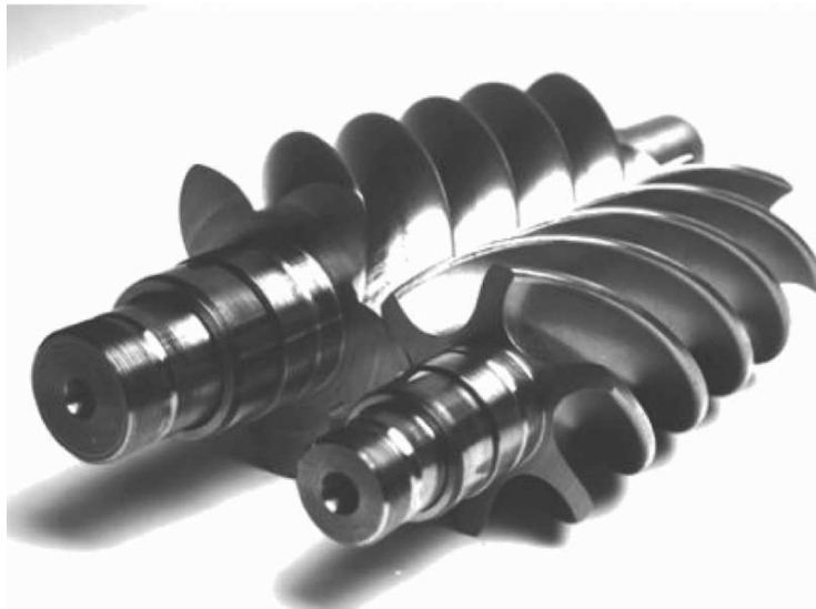
Figure 4-14 Drawing and photograph of 5/6 male and female 'N' rotors
