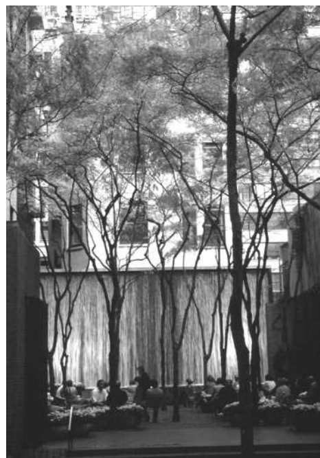
Fig. 19. Paley Park. New York City. A shaded and cooled microclimate. Waterfall creates evaporative cooling and sets up local breezes, also creating acoustic masking of street traffic.
