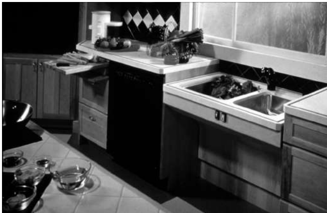
Fig. 13. G. E. Real Life Design Kitchen including adjustable height appliances and counters, natural light and high contract trim for users with low vision. Mary Jo Peterson, Interior Design.
