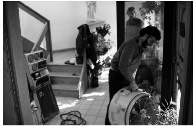
Blower door testing to check insulation and air-exchange provisions
