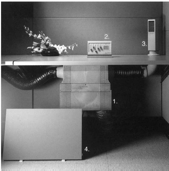
Fig. 7. Personalized Environmental Module (PEM™), developed by Johnson Controls, permits individual control of task air temperature, air speed and air direction. Key: (1) mixing box, (2) control panel, (3) desktop diffuser, (4) radiant panel.
