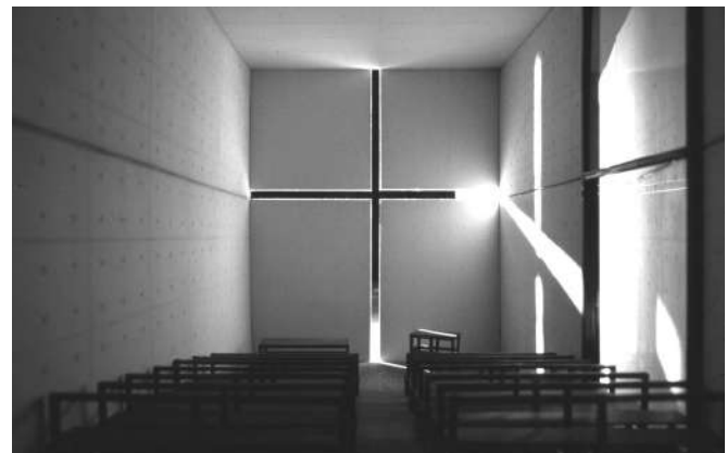
Fig. 16. Church of the Light. Osaka Prefecture. Japan. Tadao Ando, Architect. 1989. Daylight model study Hiro Ogino and Peter Sprouse. Winter solstice 9 am. Daylight factor = 2%
