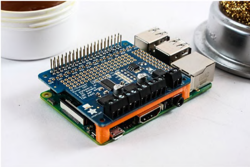
Figure 6-14. The completed board mounted on the Raspberry Pi. The orange support piece is 3D printed.
