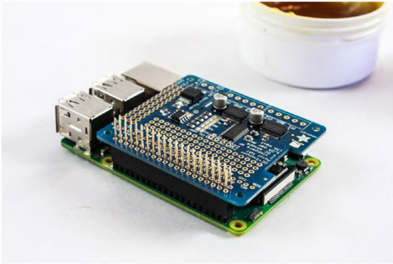
Figure 6-7. Circuit board mounted on the header
