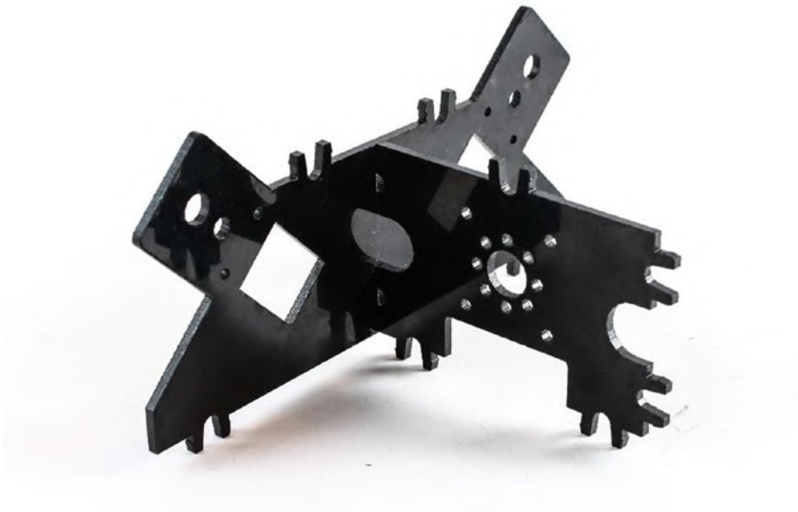
Figure 7-2. Center support attached to an outer plate
