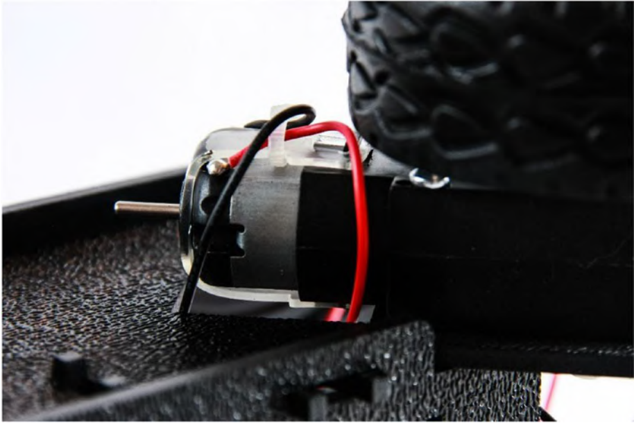
Figure 7-8. Motor wires fed through the hole behind the motor
