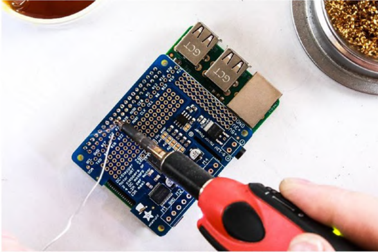
Figure 6-10. Rotate the Pi and solder the remaining pins
