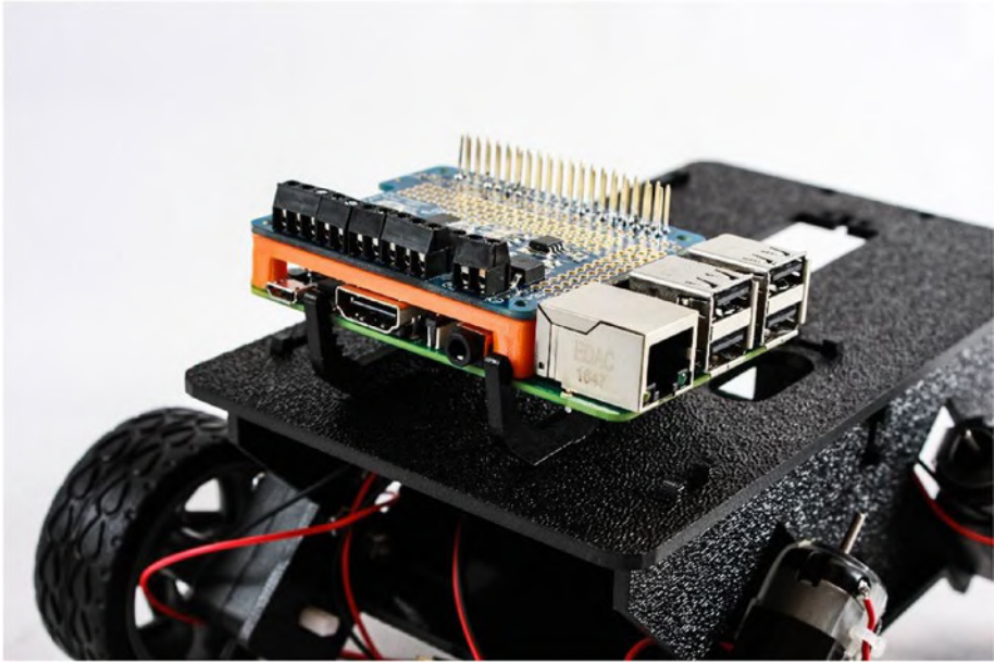
Figure 7-10. Raspberry Pi mounted in the clips
