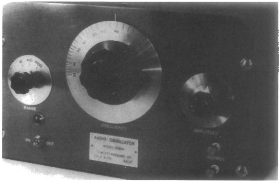
Figure 7-1. One of the original Hewlett-Packard Model 200A oscillators—the good guys won and nobody lost. (Photo courtesy of Hewlett-Packard Company.)
