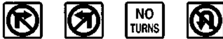
Figure 4.9: Turn Prohibition Signs (Used with permission of Federal Highway Administration, U.S. Department of Transportation, Manual on Uniform Traffic Control Devices , Millennium Edition, pg. 2B-14, Washington DC, 2000.)
