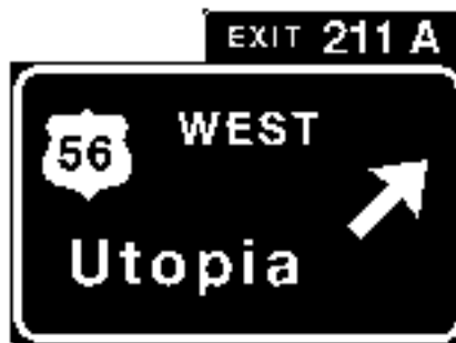
Figure 15.12: A Typical Freeway Directional Guide Sign (Used with permission of Federal Highway Administration, Manual on Uniform Traffic Control Devices , Millennium Edition, Washington DC, Figure 2F-18, pg. 2F-33.)
