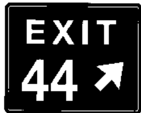
Figure 15.14: Gore Area Exit Sign (Used with permission of Federal Highway Administration, Manual on Uniform Traffic Control Devices , Millennium Edition, Washington DC, Figure 2F-19b, pg. 2F-50.)
