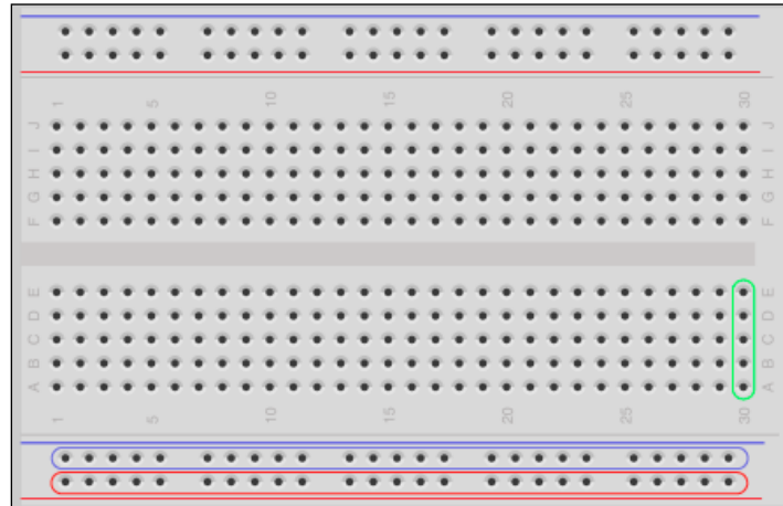
A breadboard with its buses blue and red and its numerous perforations
