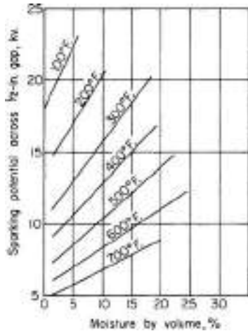
FIG. 17-65 Sparking potential for negative point-to-plane 1/2-in (1.3-cm) gap as a function of moisture content and temperature of air at 1-atm (101.3-kPa) pressure. [Sproull and Nakada, Ind. Eng. Chem. , 43, 1356 (1951).]
