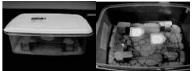
FIG. 12-12 Sorption isotherm apparatus. A saturated salt solution is in the bottom of the sealed chamber; samples sit on a tray in the headspace.
