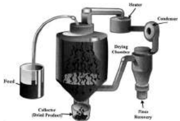
FIG. 21-173 Schematic of a typical spray-drying process. [Çelik and Wendel, in Parikh (ed.), Handbook of Pharmaceutical Granulation Technology , 2d ed., Taylor & Francis, 2005. With permission.]
