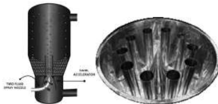
FIG. 21-170 Niro™ Precision Granulation process. Agglomeration in bottom-spray draft tube fluid-bed granulation. Scale-up is accomplished by replicating draft tube geometry. (Courtesy Niro Pharma Systems.)
