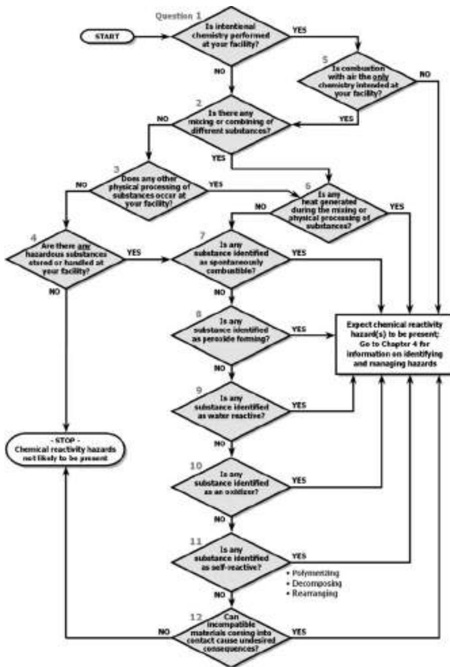
FIG. 23-18 CCPS preliminary screening for chemical reactivity hazards. [From Johnson et al. (2003); copyright AIChE; reproduced with permission.]
