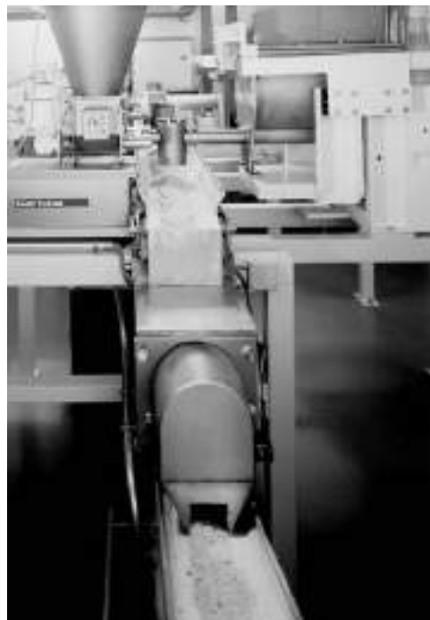
FIG. 21-54 Continuous mixing for the production of Muesli: Continuous gravimetric solids feeder (loss-in-weight feeding) supplies the components (raisins, flakes, etc.) at constant rate onto a belt, which delivers the components to the continuous mixer (bottom of the picture). The continuous mixer discharges onto a second belt.
