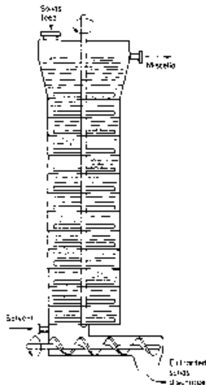
FIG. 18-88 Bonotto extractor. [Rickles, Chem. Eng. 72(6): 163 (1965); copyright 1965 by McGraw-Hill, Inc., New York. Excerpted with special permission of McGraw-Hill.]
