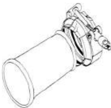
FIG. 10-166 Joint with beaded pipe ends. (Adapted with permission of De Dietrich Process Systems, Mountainside, N.J.)
