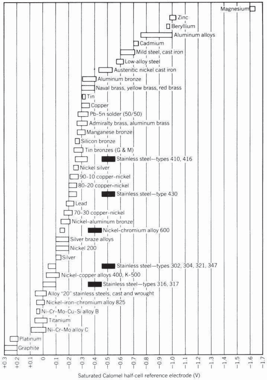
Figure 2 Corrosion potentials in flowing seawater (8–13 ft/s), temperature range 50–80°F. Alloys are listed in the order of the potential they exhibit in flowing seawater. Certain alloys, indicated by solid boxes, in low-velocity or poorly aerated water and at shielded areas may become active and exhibit a potential near -0.5 V.
