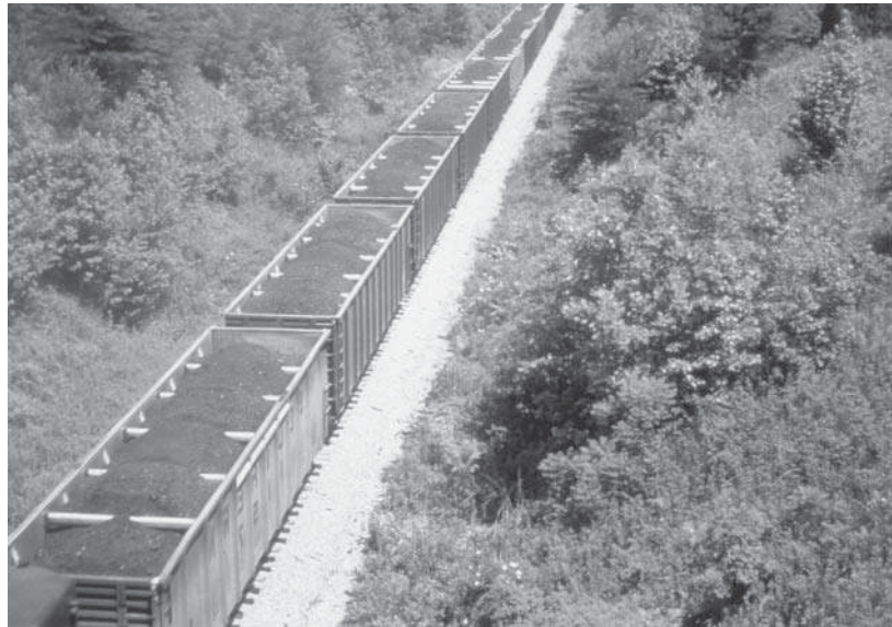
Figure 10 Alloy 5454 has been widely used for railcar body construction where heavy loads, such as coal, and potentially high temperatures may be involved. (Courtesy of the Aluminum Association.)
