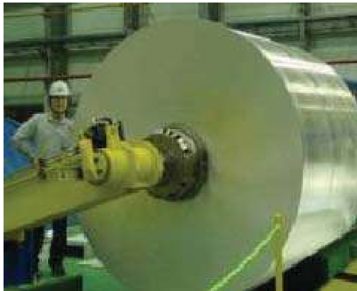
Figure 1 Twin roll cast magnesium alloy strip cast coil, 2000 mm wide. 5
