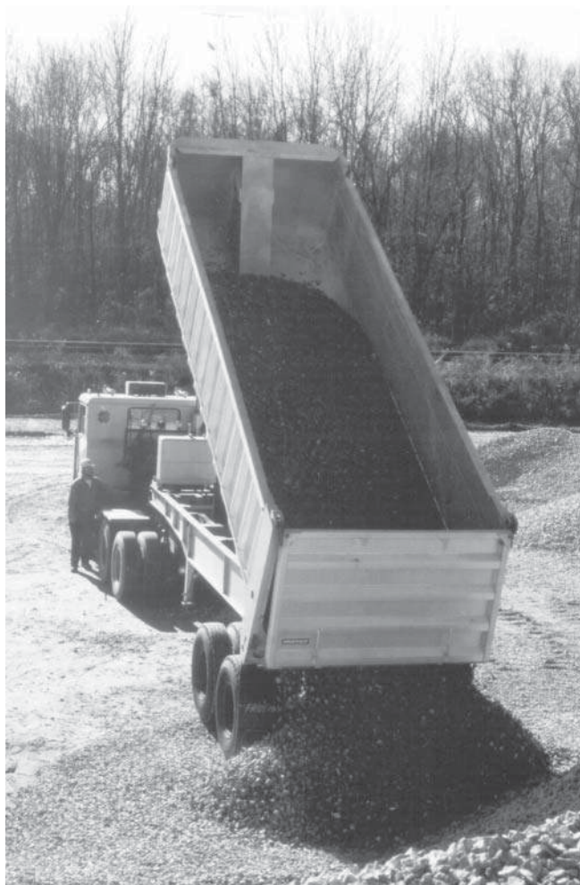
Figure 4 Heavy dump and tank trucks and trailer trucks employ high-strength 2xxx or 6xxx extrusions for their structural members and tough 5xxx alloy sheet and plate for their load-carrying components. (Courtesy of the Aluminum Association.)
