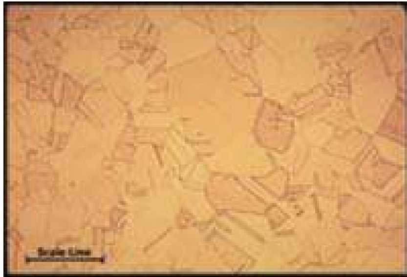
Figure 1 Microstructure of pure copper. Courtesy of The Copper Development Association, Inc.
