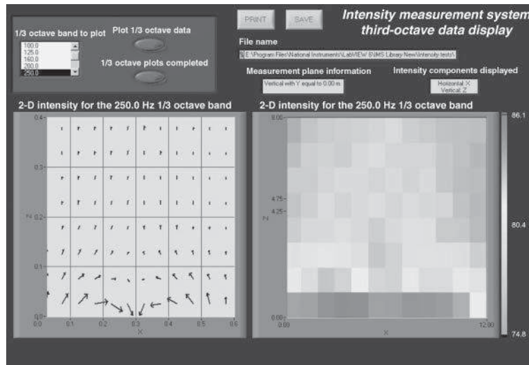
Figure 23 Graphical display of an automated sound intensity measurement system developed for NASA Glenn Research Center.
