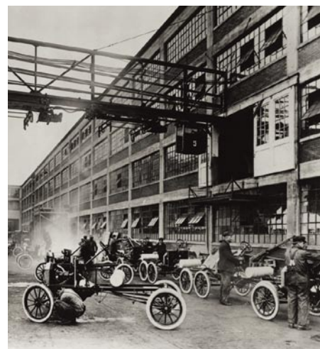
▲ The Model T Ford was available “in any color as long as it’s black”. Black was the only color of paint that would dry quickly enough to keep up with the production line seen here.
