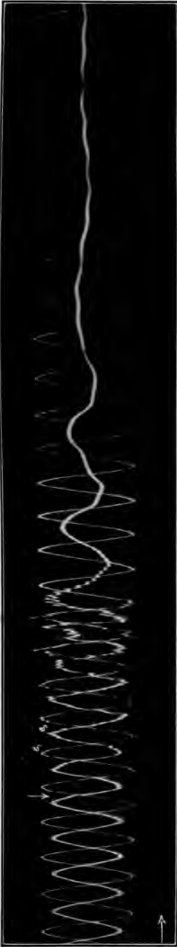
Fig. 48B. — cd 10049. — Oscillogram of High-frequency Oscillation Preceding Low-frequency Oscillation of Compound Circuit Caused by Switching 154 miles of 100,000 Volts Transmission Line and Step-down Transformer off another 154 Miles of 100,000 Volts Line; High-tension Switching.
