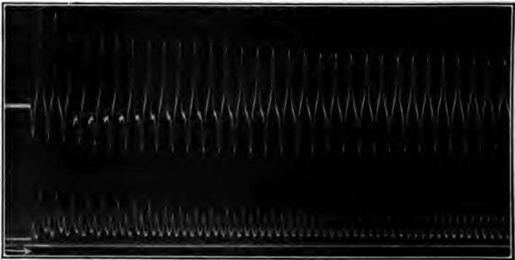
Fig. 28. — cd6565. — Asymmetrical. Momentary Single-phase Short Circuit of 5000-Kw. 11,000-Volt Three-phase Alternator ( ATB-6-5000-500 ). Oscillogram of Armature Current and Field Current.
