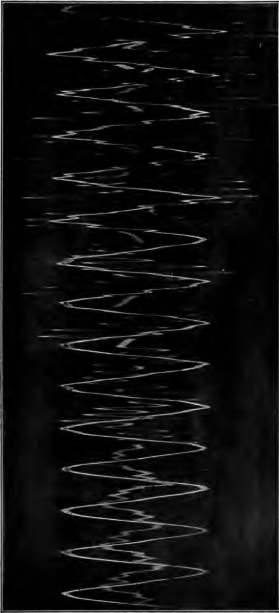
Fig. 46. — cd10001. — Oscillogram of Cumulative Oscillation in High-potential Coil of 2500-kw. Step-up Transformer Caused by Disconnecting 28 Miles of 100,000-volt Transmission Line; High-tension Switching.
