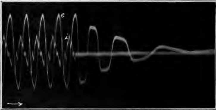
Fig. 31.—CD10017.—Oscillogram of Stationary Oscillation of Varying Frequency: Compound Circuit of Step-up Transformer and 28 Miles of 100,000-volt Transmission Line.
