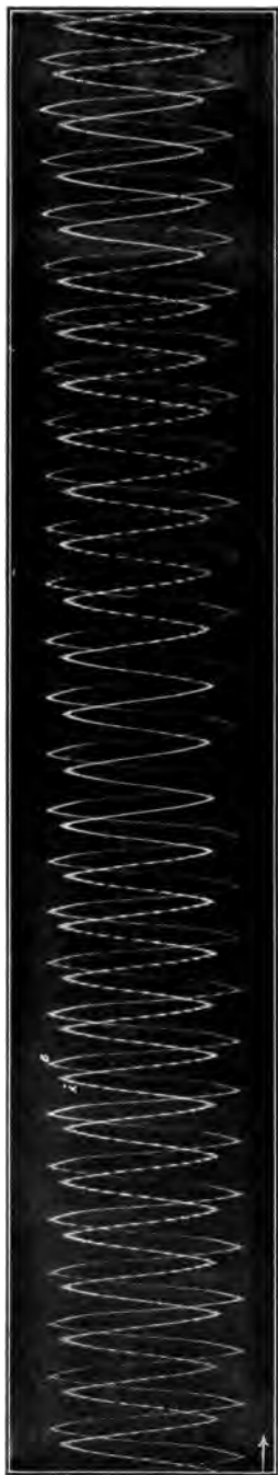
Fig. 44. — cd10057. — Oscillogram of Beginning of Arcing Ground on 154 Miles of 100,000-volt Transmission Line.
